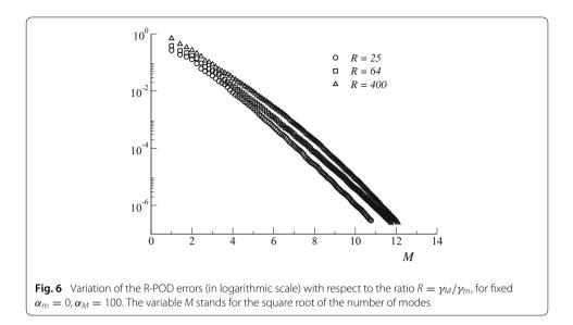
history for Data 3, computed for R = 25, 64 and 400, in all cases with a fixed interval of reaction rates  $[\alpha_{m}, \alpha_{M}] = [0, 100]$ , with respect to the square root of the numbers of modes,  $M = \sqrt{L}$ . We can point out that the convergence rate degrades as *R* increases, in accordance with the fact that
