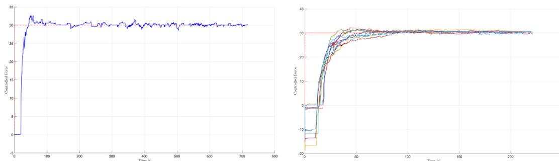
Figure 8: **Left.** Long-term experiment to verify the asymptotic stabilization of the grasping - Force ( $N$ ) versus time ( $sec$ ). **Right.** 10-time experiments to highlight the efficiency and the repeatability of the grasping - Force ( $N$ ) versus time ( $sec$ ).
