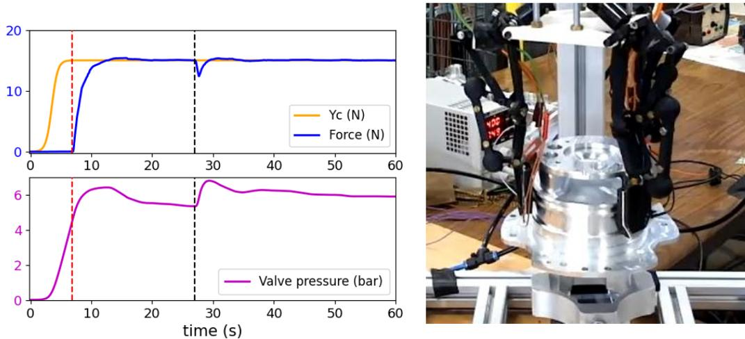
Figure 5: **Scenario 1.** **Left top.** Desired (yellow) and real (black) forces ( $N$ ) versus time (sec). **Left bottom.** Pressure (bar) versus time (sec). **Right.** Photo of the experimental set-up with a spherical grip.
