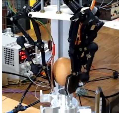
Figure 6: Scenario 2. Left top. Desired (yellow) and real (black) forces ( N ) versus time (sec). Left bottom. Pressure (bar) versus time (sec). Right. Photo of the experimental set-up with a prismatic grip.
