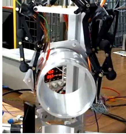
Figure 6: Scenario 2. Left top. Desired (yellow) and real (black) forces ( N ) versus time (sec). Left bottom. Pressure (bar) versus time (sec). Right. Photo of the experimental set-up with a prismatic grip.
