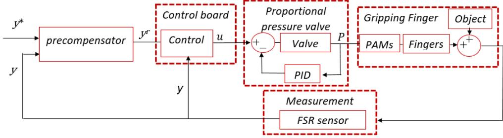
Figure 2: Closed-loop scheme including a pre-compensation of the desired trajectory:  $y$  is the measured force,  $y^*$  is the desired reference trajectory, and  $y^r$  is the reference trajectory defined by (1).
