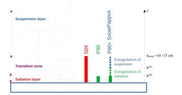
**Figure 1.** Schematic representation of the suspension and saltation layers and of the transition zone between them. The fluxes computed by the two saltation models S04 and P90 are represented schematically, as well as the "P90 + SnowPappus" method, combining the P90 saltation model and the SnowPappus suspension model.
