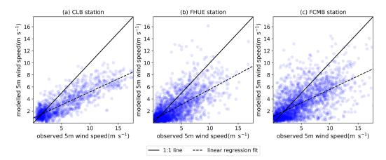
**Figure 10.** Comparison between observed wind at Col du Lac Blanc as well as at Huez and Chambon ISAW stations and the 250 m resolution DEVINE-modelled wind used as a forcing in the closest simulation points. Linear regression lines fitting the modelled wind as a function of the observed ones are presented. The presented points are the ones used for blowing-snow occurrence evaluation in Fig. 9. Wind observed data were filtered using the same algorithm as in Le Toumelin et al. (2022).
