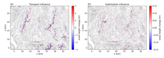
**Figure 12.** (a) Snow depth difference (m) between the TRANS and CTRL simulation on 16 March 2018, which approximately corresponds to the end of the accumulation season. (b) Snow depth difference (m) between TRANS+SUBL and TRANS simulations.
