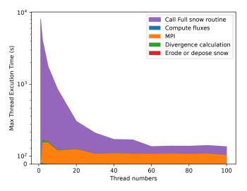
**Figure A3.** Visualization of the maximum thread execution time spent in the different parts of SnowPappus (named as in Fig. 4) and spent in the other snow routines. This time is mainly dedicated to running the Crocus snow model.
