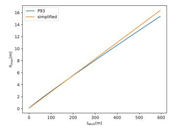
**Figure A2.** Comparison between the height  $h_{\text{max}}$  given in Sect. 3.3.2 used as an upper bound for suspension transport (blue curve) and the one computed with Eq. (10) from Pomeroy et al. (1993) (orange curve). Both heights are plotted as a function of the fetch distance as defined in Sect. 3.3.2.
