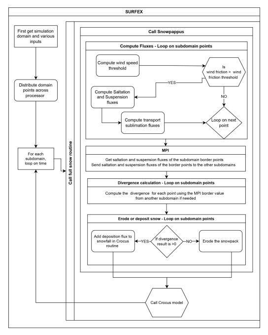
Figure 4. Description of how the SnowPappus routine is organized in the SURFEX framework and how it connects with the Crocus snow model.
