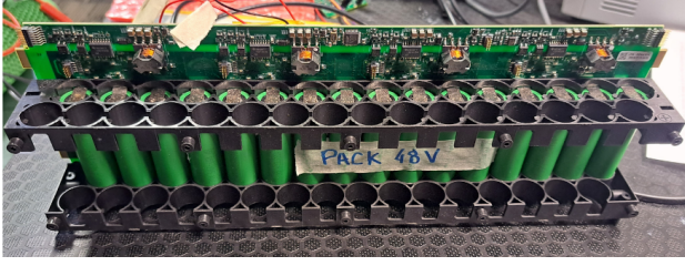
Fig. 1. The 48V pack with 16 cells.
