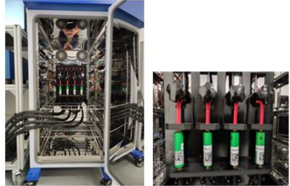
Fig. 3. The tests on the 4 cells of Sony VTC6
