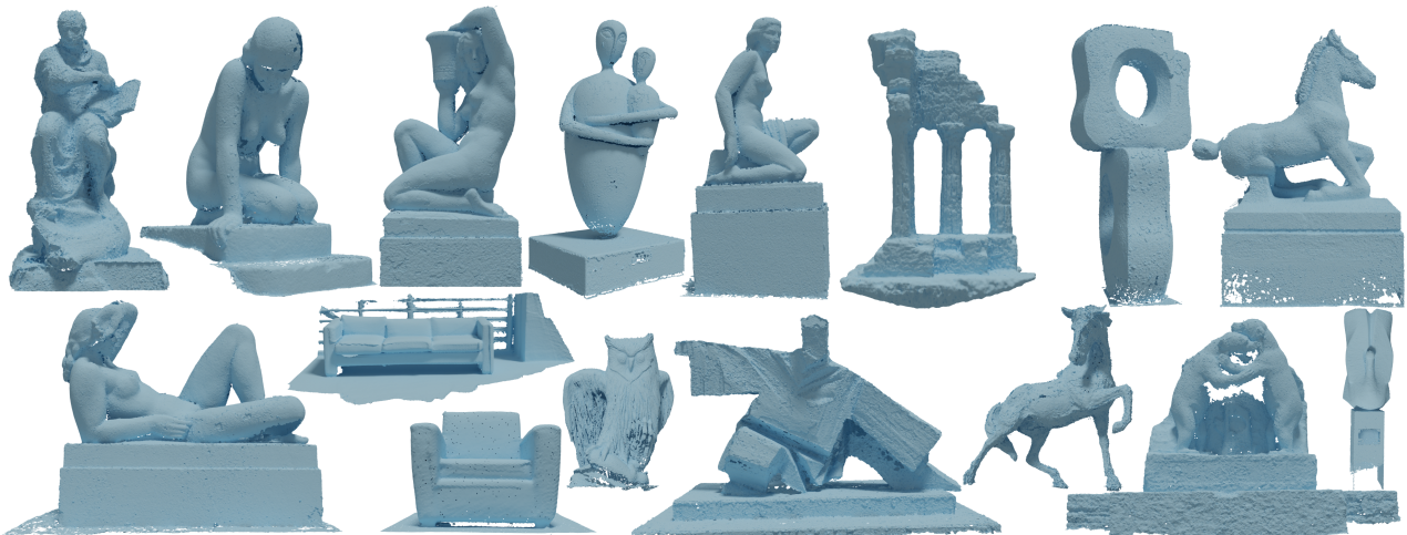
Figure 26: Meshes generated via LOCAL BALLMERGE (with default \delta = 1.85 and \eta = 200 ) of real-world point clouds (up to 1378k points) from the KSR42_dataset [BL20] and the Statue Model Repository (©EPFL Geometric Computing Laboratory).
