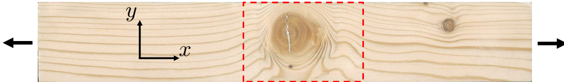
Figure 7: Wood specimen tested in this study. The red rectangle approximately corresponds to the zone over which the checkerboard patterns are deposited in turn, and thus strain maps are obtained. See the following figures where those maps are displayed after anticlockwise rotation of this zone by 90 degrees.
