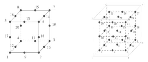
Figure 6. C3D20R elements with corresponding integration points [12].
