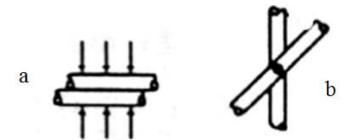
Figure 8. Contact mode in the conductor: (a) lineic, (b) tangential [12].
