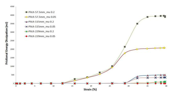
Figure 24. Frictional dissipated energy versus pitch length and friction coefficient.
