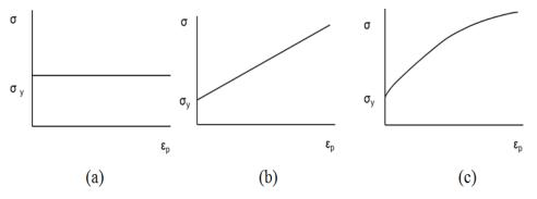
Figure 2. Hardening laws: (a) Perfect plasticity; (b) Linear hardening; (c) Non-linear hardening [12].
