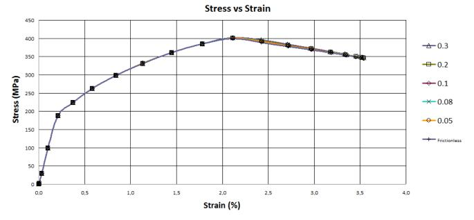
Figure 11. Stress-strain for various friction coefficients.
