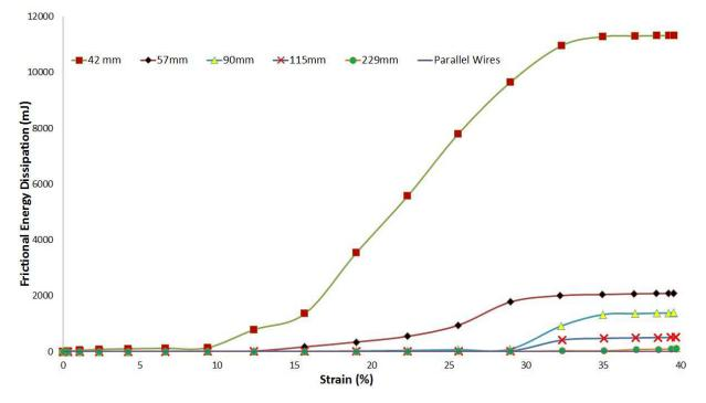
Figure 23. Frictional dissipated energy variation versus pitch length.
