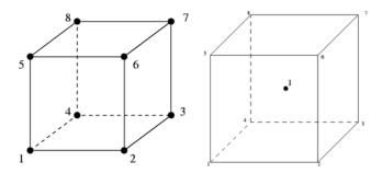
Figure 5. C3D8R Elements with an integration point [12].
