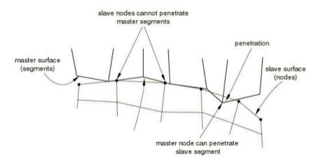
Figure 9. Rules of penetration of slave/master nodes [12].
