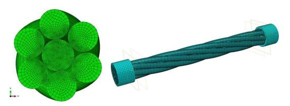
The elements of contact areas were refined. In total, the problem to be solved is composed of 25252 nodes and 23026 elements (Figure 7).
