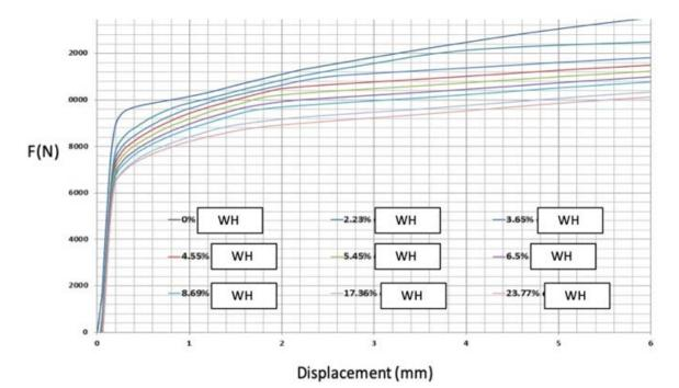
**Figure 26.** Work-hardening effect on the conductor with a 5% defect on the core wire (WH refers to Work-Hardening).
