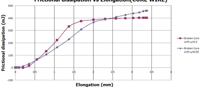
Frictional dissipation vs Elongation(CORE WIRE)
