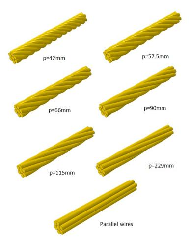
Figure 19. Conductor types with various pitch.
