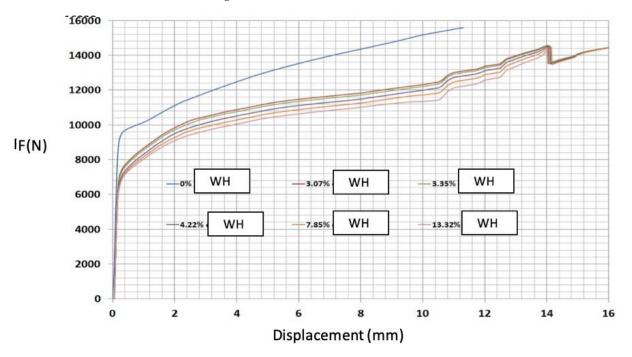
**Figure 27.** Work-hardening vs. the behavior of the phase with 10% local defect at the core wire (WH refers to Work-Hardening).
