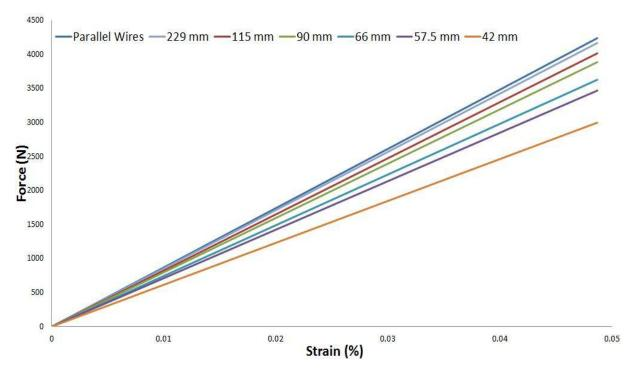
Figure 22. Conductor elastic area versus pitch length (analytical results).
