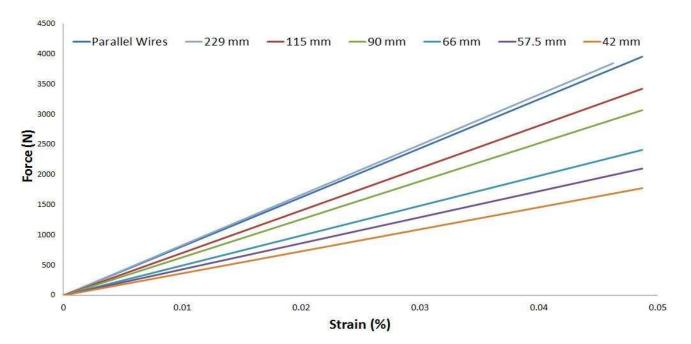
Figure 21. Variation of the elastic part of copper versus the pitch length (numerical results).
