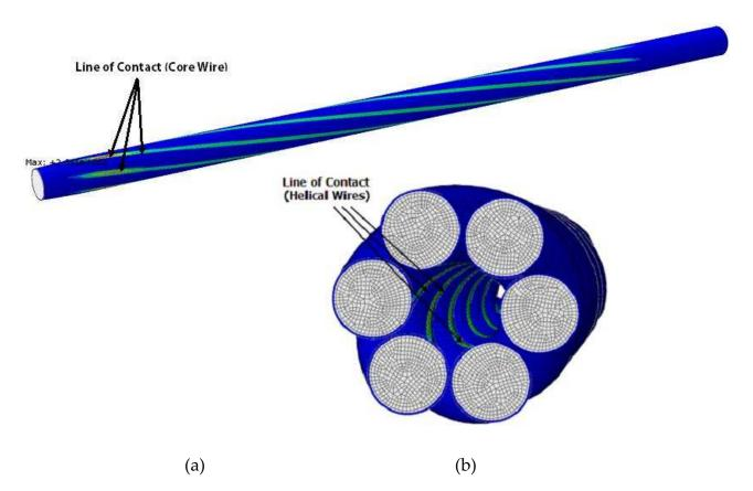
Figure 13. Contact line at the core-wire (a) and at the helical wire (b).
