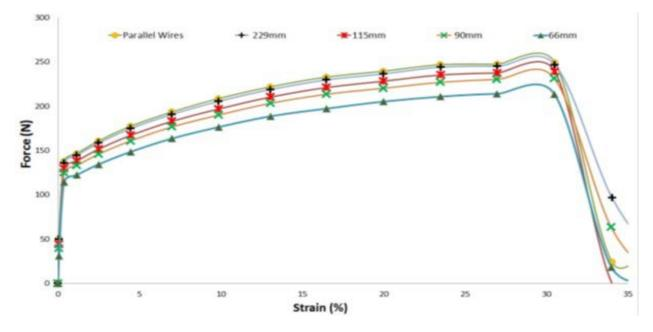
Figure 20. Simulated mechanical behavior of copper for various pitch values.
