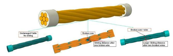
Figure 18. Various cases studied (healthy conductor), core-wire broken, one helical wire broken).
