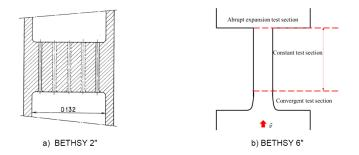
Figure 6: Diagram of the two test sections of the BETHSY experiment.
