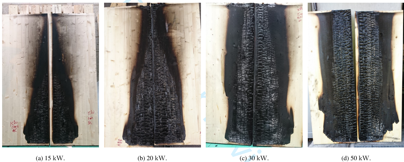
Figure 5: Photos of test specimens after 15 minutes of testing with burner powers ranging from 15 to 50 kW.
