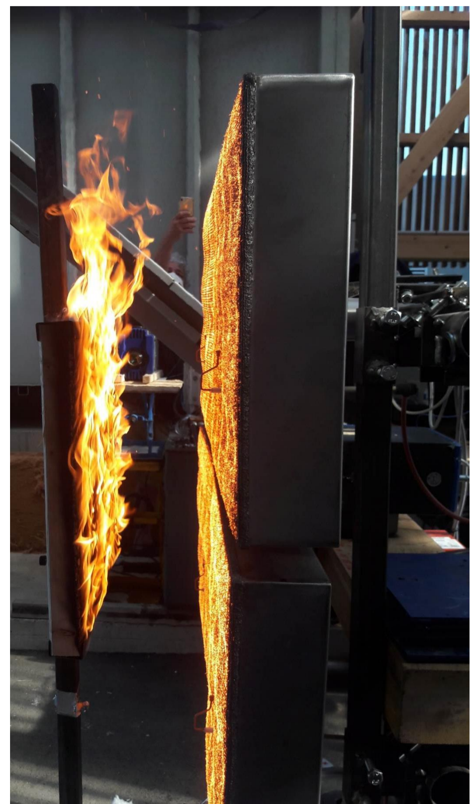
Fig. 1. Wood sample exposed to 60 kW.m -2 .
