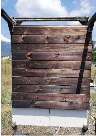
Fig. 7. Wood cladding after the test 3.
