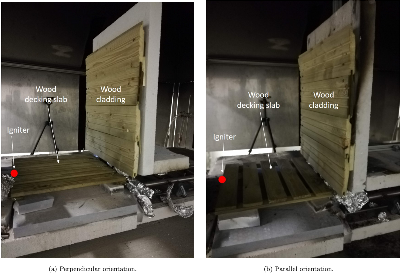
Figure A.15: Orientation of wooden decking slabs for a vertical distance of 2 cm between the cladding and the slab.
