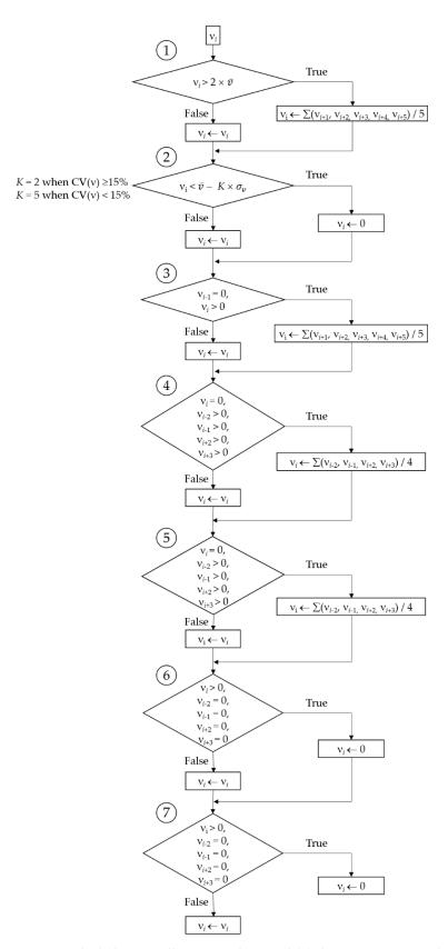
**Figure 1.** Block diagram illustrating the speed (v) data processing methodology.  $\overline{v}$ ,  $\sigma_v$ , CV(v) are the mean, standard deviation, and coefficient of variation of speed over the representative 120-s (or shorter if not possible) period of the session; vi is the speed value corresponding to the epoch i. At each of the seven steps, vi outputs  $(vi \leftarrow)$  are new values that are included in a new vector v.
