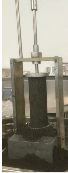
Figure 11. Cutting device for the soil samples. Alt Text: Photograph of the cutting device of the soil samples.
