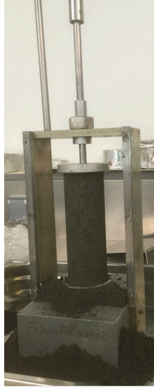
Figure 11. Cutting device for the soil samples. Alt Text: Photograph of the cutting device of the soil samples.
