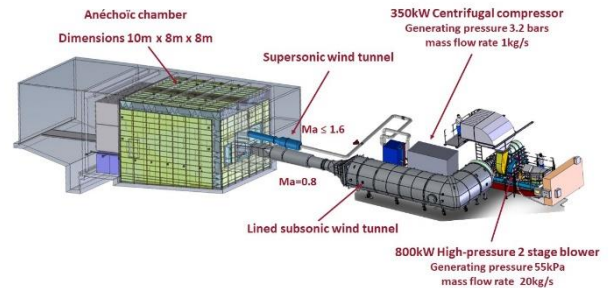
Figure 4. 3D schematic view of the main experimental facility of the Acoustic Center (blower and compressor, wind tunnels and anechoic chamber).
