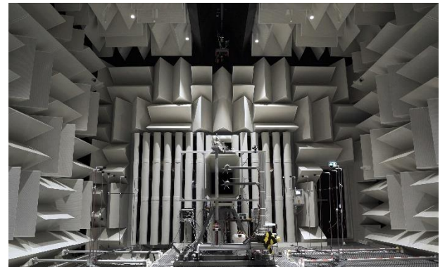
Figure 5. Internal view of the anechoic chamber and of the exhausts of the subsonic and supersonic wind tunnels.
