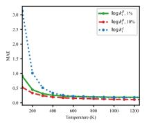
**Fig. 5.** Mean absolute error of the predictions (using the 8 features) for 1% (green solid line) and 10% (red dashed line) of the full dataset used for the training, compared to the QCT results (blue dotted line), as functions of the temperature.
