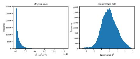
**Fig. 2.** Histogram of the labels  $k_i^q$ , the accurate rate constant with *i* representing a given rovibrational transition, before and after transformation. We apply a Yeo-Johnson transform [37] the negative of the logarithm with base 10 of the original  $k_i^q$  labels. The transformed data have zero-mean and unit-variance.
