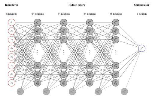
**Fig. 1.** Our multilayer perceptron architecture MLP1, composed of 4 hidden layers of 64, 64, 64 and 48 neurons each and 8 features,  $x_1...x_8$ , for the input neurons and one output neuron,  $y^p$ . Bias neurons,  $w_0^{(L)}$  connected to the hidden layers, and to the output layer, L = 6, are represented. We also use in this work another multilayer perceptron, MLP2, of 4 hidden layers of 32, 48, 64 and 64 neurons each, with only 7 features.
