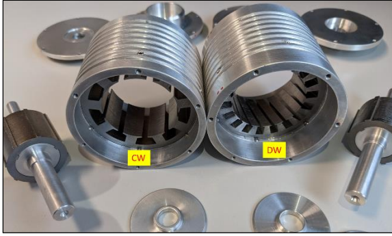
Fig. 7: DW and CW prototypes without winding and magnet
