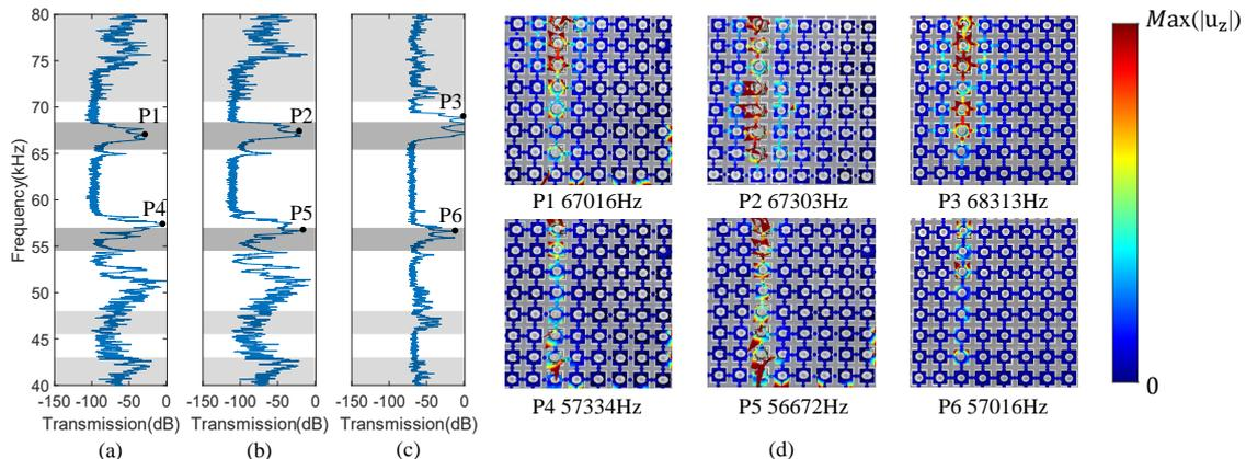
Figure 5: Measured transmissions of the straight waveguides with different torques: (a)  $2.3 \text{ N} \cdot \text{m}$ , (b)  $2.7 \text{ N} \cdot \text{m}$ , and (c)  $3.0 \text{ N} \cdot \text{m}$ . Vibration modes at the corresponding labeled points are given in panel (d). The color scale represents the normalized amplitude of out-of-plane displacements from 0 (blue) to maximum (red).
