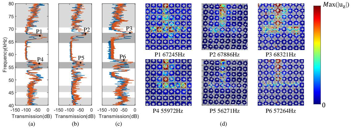
Figure 9: Measured transmissions of the wave splitter with different torques: (a)  $2.3 \text{ N} \cdot \text{m}$ , (b)  $2.7 \text{ N} \cdot \text{m}$ , and (c)  $3.0 \text{ N} \cdot \text{m}$ . Transmissions measured on the right and left outputs are marked by blue and red, respectively. Vibration modes at the corresponding labeled points are given in panel (d). The color scale represents the normalized amplitude of out-of-plane displacements from 0 (blue) to maximum (red).
