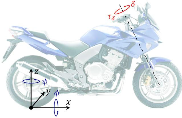
Fig. 1. The coordinate system used in this study, showing the positive directions for roll  $\phi$  and yaw  $\psi$  motions. The positive direction for the steering angle  $\delta$  and the steering torque  $\tau_\delta$  is also shown.
