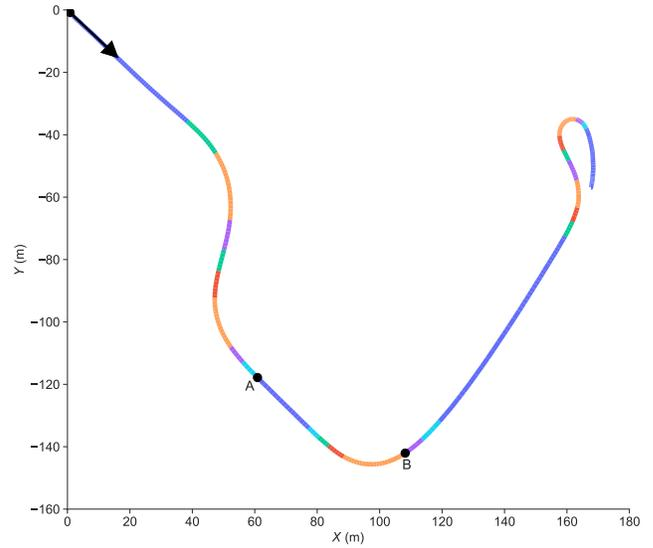
Fig. 3. Trajectory of the trial divided into segments. The colour of each segment indicates the cluster it belongs to: VR (Vertical Riding); SC (Steady Cornering); LIF (Lean-In Fast); LOF (Lean-Out Fast); LIE (Lean-In End); ALD (Accelerating in Lean Direction). The arrow indicates the direction of travel. Letters A and B delimit the corner entry manoeuvre analysed.
