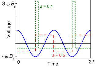
Fig. 2. Example of investigated voltage waveforms for given peak induction  $B_{\rm P}$ : sinusoidal, symmetric square, and asymmetric square with duty cyle a = 0.1.
