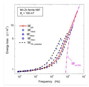
Fig. 12. Same as Fig. 11 for the Mn-Zn ferrite. Besides the loss under triangular symmetric induction  $W_{\text{TRIOS}}(f)$ , the same quantity for asymmetric induction, with duty cycles  $a = 0.2 (W_{\text{TRIO2}}(f))$  and  $a = 0.1 (W_{\text{TRIO1}}(f))$  is measured (symbols) and predicted (dashed lines), starting from the loss components of  $W_{\text{SIN}}(f)$  and applying (7).
