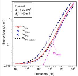
Fig. 11. The broadband (DC - 1 MHz) energy loss behavior at  $B_p = 100$  mT under triangular symmetric ( $W_{\text{TRI05}}$ ) and asymmetric ( $W_{\text{TRI01}}$ , duty cycle a = 0.1) induction, measured in the nanocrystalline Finemet transverse anisotropy tapewound ring sample (symbols), is compared with the same quantity  $W_{\text{SIN}}(f)$  (line and symbols) measured with sinusoidal induction. By making the loss decomposition of  $W_{\text{SIN}}(f)$  are predicted (dashed lines).
