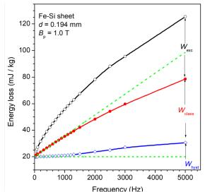
Fig. 6. As in Fig. 5 for the 0.194 mm thick non-oriented Fe-Si sheets. The components  $W_{hysl}(f)$  and  $W_{el,SIN}(f)$  are calculated using (12) and (13). The effect of the frequency dependent non-uniform induction profile becomes apparent beyond about 1500 Hz, where the conventional prediction disregarding the skin effect (dashed lines) departs from the abovementioned calculation.
