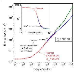
Fig. 3. Broadband behavior of energy losses at  $B_p = 100$  mT in the tapewound transverse anisotropy ( $K_{\perp} = 25$  J/m<sup>3</sup>) Finemet-type nanocrystalline ribbon and in the N87 Mn-Zn ferrite.  $d \equiv$  thickness,  $\langle s \rangle \equiv$  average grain size. Symbols: fluxmetric measurements. Solid lines: measurements by transmission line and VNA and use of (2). The inset shows the corresponding frequency dependence of the real relative permeability  $\mu'r$ .
