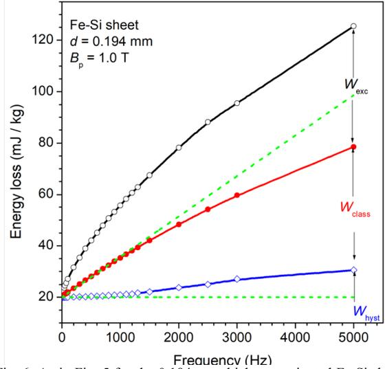
Fig. 6. As in Fig. 5 for the 0.194 mm thick non-oriented Fe-Si sheets. The components  $W_{\text{hyst}}(f)$  and  $W_{\text{cl,SIN}}(f)$  are calculated using (12) and (13). The effect of the frequency dependent non-uniform induction profile becomes apparent beyond about 1500 Hz, where the conventional prediction disregarding the skin effect (dashed lines) departs from the abovementioned calculation.
