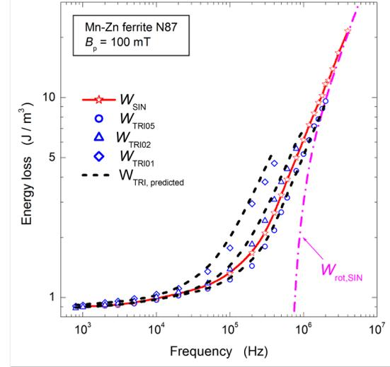
Fig. 12. Same as Fig. 11 for the Mn-Zn ferrite. Besides the loss under triangular symmetric induction  $W_{\text{TRI05}}(f)$ , the same quantity for asymmetric induction, with duty cycles  $a = 0.2$  ( $W_{\text{TRI02}}(f)$ ) and  $a = 0.1$  ( $W_{\text{TRI01}}(f)$ ) is measured (symbols) and predicted (dashed lines), starting from the loss components of  $W_{\text{SIN}}(f)$  and applying (7).
