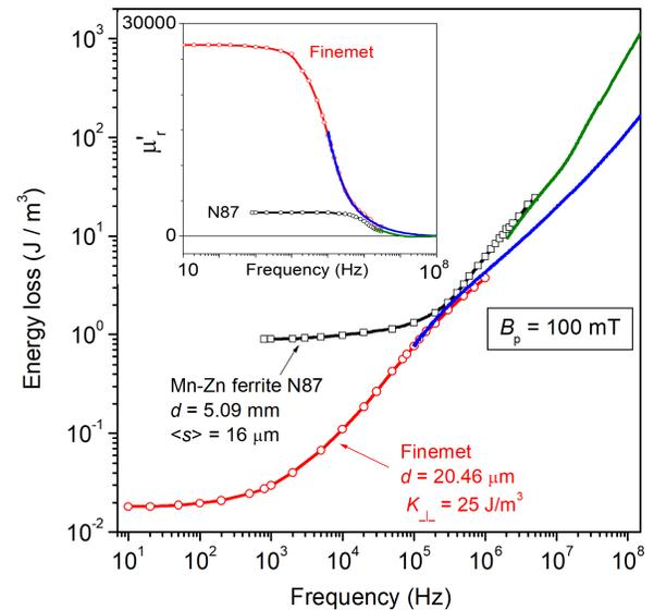
Fig. 3. Broadband behavior of energy losses at  $B_p = 100$  mT in the tapewound transverse anisotropy ( $K_{\perp} = 25$   $\text{J/m}^3$ ) Finemet-type nanocrystalline ribbon and in the N87 Mn-Zn ferrite.  $d \equiv$  thickness,  $\langle s \rangle \equiv$  average grain size. Symbols: fluxmetric measurements. Solid lines: measurements by transmission line and VNA and use of (2). The inset shows the corresponding frequency dependence of the real relative permeability  $\mu_r$ .
