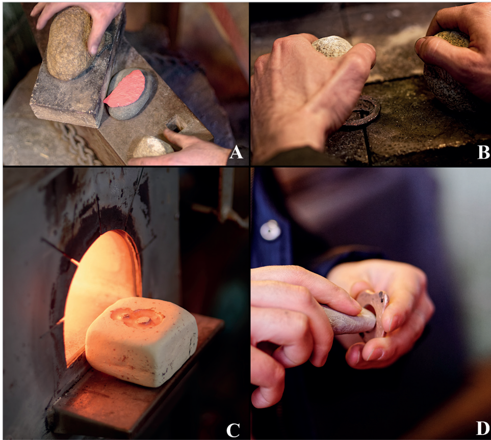
Fig. 2a. Hot hammering of a “copper pebble” fragment; 2b. Cold hammering of a “ring idol” pre-shape; 2c. Casting in an open mould; 2d. Abrasive work and polishing (photographs by N. Gilbert).
