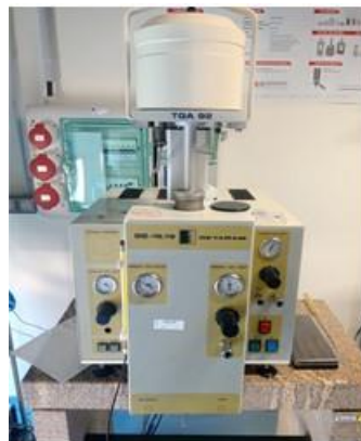
Fig. 2. The thermobalance used to carry out the oxidation tests.
