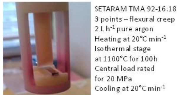
Fig. 3. The creep sample before introduction in the furnace and the application of the constant force.
