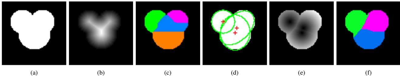
**Fig. 4:** (a) Illustration of overlapping nuclei. (b) Application of the classic Euclidean distance transform to the nuclei. (c) Resulting watershed segmentation derived from the maximum intensity peaks of the Euclidean distance transform. (d) Distance Transform Ellipse Center Method Algorithm (DTECMA). (e) Distance transform to the nearest ellipse center as obtained from DTECMA. (f) Watershed segmentation resulting from the DTECMA approach.
