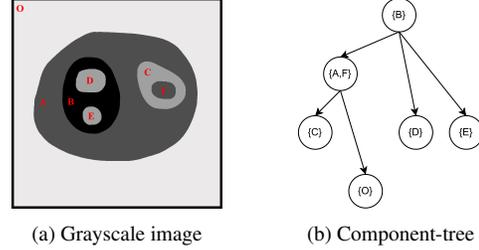
**Fig. 2:** The component-tree (b) of a grayscale image (a). Individual nodes correspond to connected components at specific gray levels, while links between nodes represents the inclusion relations between the corresponding flat zones.
