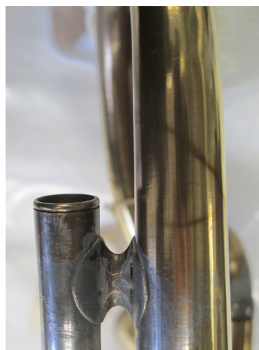
Figure 5. Silver corrosion due to a Nacrylan thread
