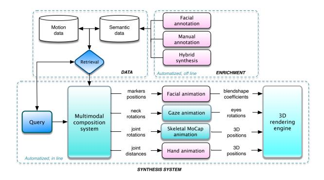
Fig. 1. Text-to-SL SignCom synthesis system with signing avatar. In blue: basic system [1]. In pink: advanced technological modules
