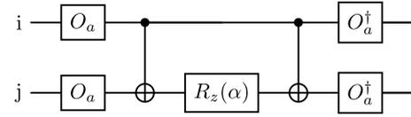
FIG. 10. Quantum circuit decomposition of the unitary operator  $e^{-i\frac{\alpha}{2}\sigma_i^a\sigma_j^a}$  with  $a \in \{x, y, z\}$ . Here  $i$  and  $j$  denote qubit indices, and the vertical lines represent the two-qubit CNOT gates, for which the control qubit is indicated by the black dot. The other rectangles represent one-qubit gates explicitly mentioned in Eqs. (B3).
