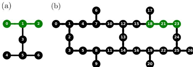
FIG. 2. Coupling map of (a) `ibmq_lagos` and (b) `ibmq_ehningen` machines. Links represent the physical junctions on which two-qubit gates can be realized. The green qubits are used for the simulation and black qubits are the idle qubits.
