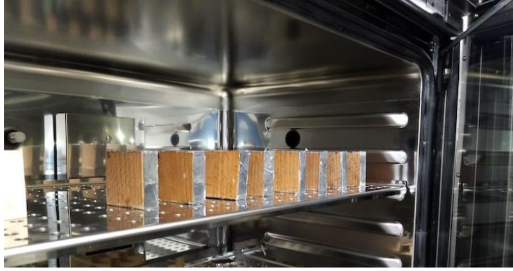
Figure 2. The climate chamber used for the drying tests in with the exchange surfaces of the samples exposed along the fan flow.
