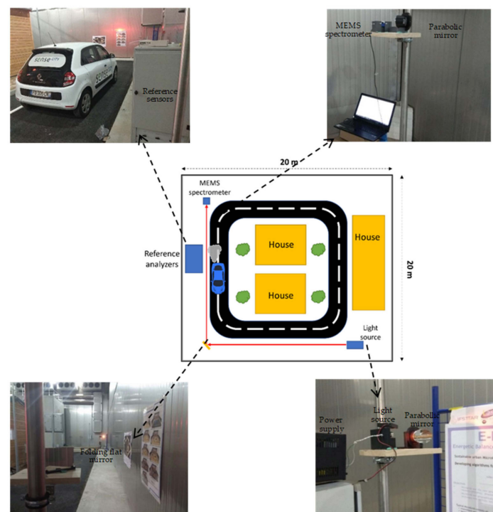
Figure 3. Top schematic view of Sense City for air pollution monitoring using open-path FTIR in addition to camera photos at different positions inside the city.
