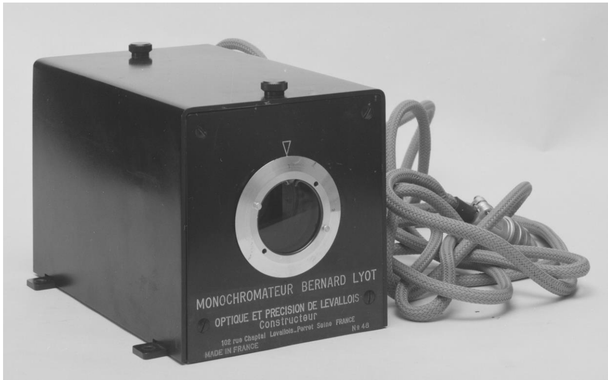
Figure 3 : the Lyot OPL birefringent monochromatic filter. The electric cable goes to the external thermostat (not shown). Courtesy OP.
