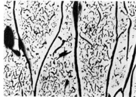
Figure 6.5. Change of the inter-lamellar spacing of the austenite/graphite eutectic. Dots and crosses are from Hillert and Rao [HIL68] and squares from Jones and Kurz [JON80, JON81]. The micrograph illustrates lamellar and undercooled graphite forms growing side by side in a directionally solidified sample (the growth direction is upwards) [HIL68].
