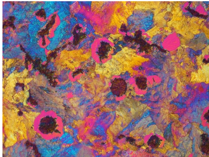
Figure 9.20. Polarized light micrograph of a pearlitic CGI.
