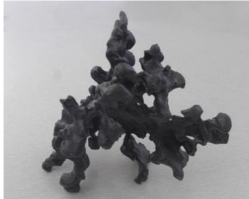
Figure 7.13. Photograph of a 3D printing of graphite in a compacted graphite eutectic cell. The model was built from a tomographic study [CHU15].
