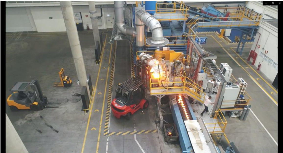
Figure 1.14. View from above of the pouring of cast iron in a modern and clean sand-mould semi-automatic line (credit: Sakthi foundry, Portugal).
