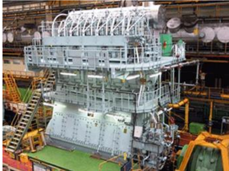
Figure 1.9. A large ship engine (Wärtsilä X62 engine). The steps on the left side can be used for an estimate of the scale. ( https://www.wartsila.com/media/news/08-01-2015-wartsila-x62-engine-now-fully-approved-and-available-to-the-market ).
