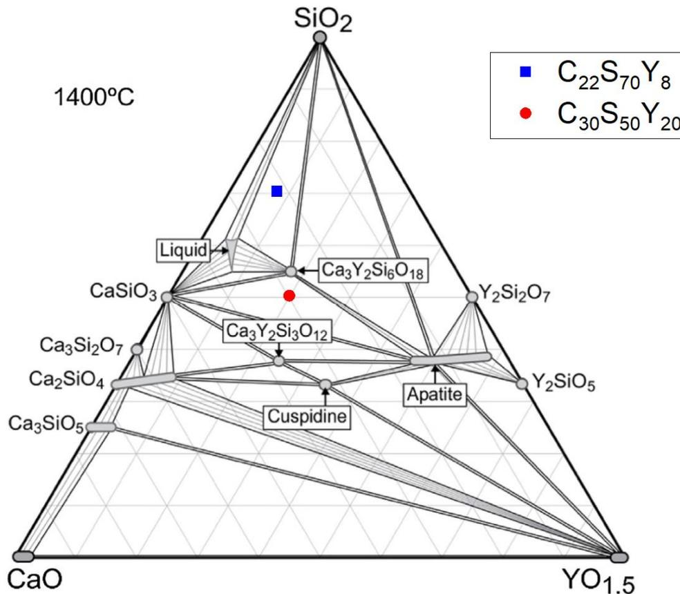
**Figure 1.** Compositions of the two systems  $C_{22}S_{70}Y_8$  and  $C_{30}S_{50}Y_{20}$  chosen for this work represented on the isotherm section à 1400°C of the  $CaO-SiO_2-YO_{1.5}$  phase diagram proposed by Poerschke et al. [9]
