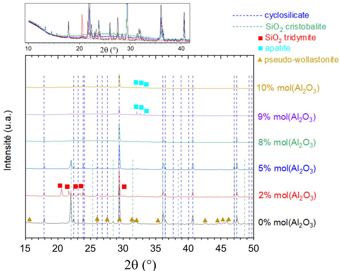
**Figure 2.** X-ray diffraction pattern of  $C_{22}S_{70}Y_8$  with addition of alumina from 0 to 10 mol.% after heat treatment at  $1300^\circ C$  for 260 hours. The diffractograms in the insert correspond to the samples with alumina addition from 0 to 8 mol.% without subtraction of the background.
