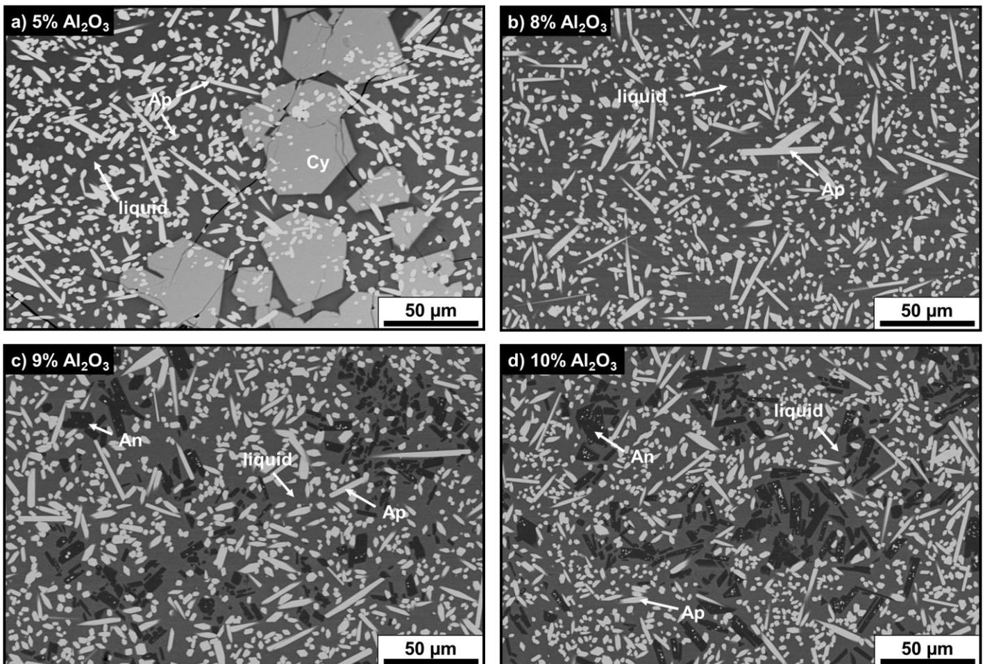
**Figure 9.** SEM micrographs (Back Scattered Electrons mode) of  $\text{C}_{30}\text{S}_{50}\text{Y}_{20}$  samples with addition of 5 mol.% (a), 8 mol.% (b), 9 mol.% (c) and 8 mol.% (d) of alumina after heat treatment at  $1300^\circ\text{C}$  for 260 hours.
