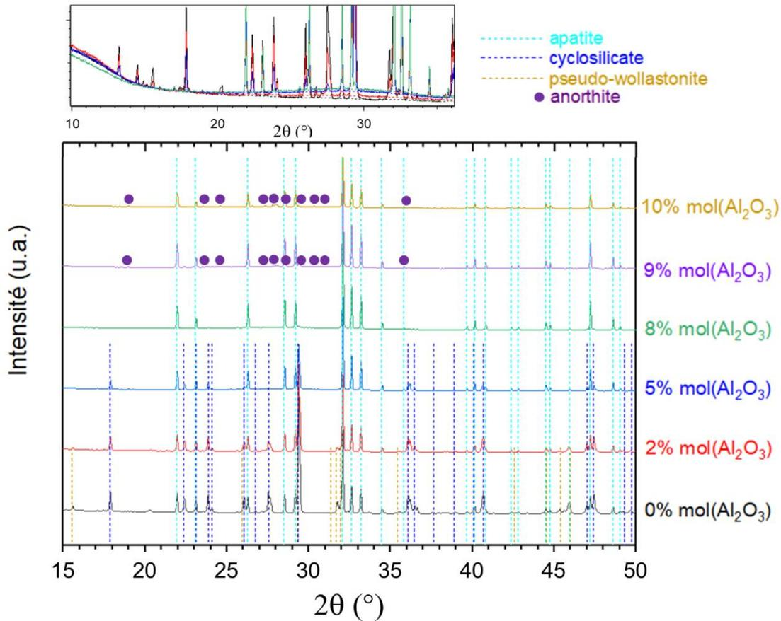
**Figure 7.** X-ray diffraction pattern of  $C_{30}S_{50}Y_{20}$  with addition of alumina from 0 to 10 mol.% after heat treatment at 1300°C for 260 hours. The diffractograms in the insert correspond to the samples with alumina addition from 0 to 8 mol.% without subtraction of the background.
