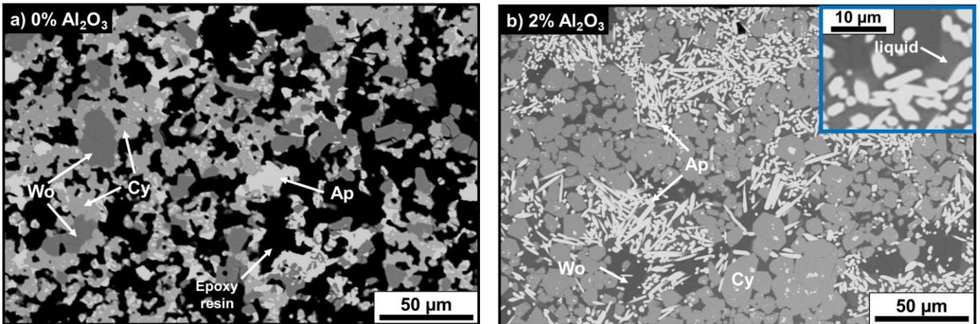
**Figure 8.** SEM micrographs (Back Scattered Electrons mode) of  $\text{C}_{30}\text{S}_{50}\text{Y}_{20}$  samples without addition of alumina (a), and with addition of 2 mol.% (b) of alumina after heat treatment at  $1300^\circ\text{C}$  for 260 hours.
