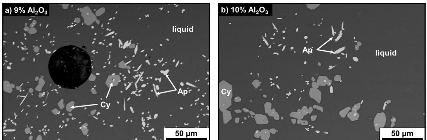
**Figure 4.** SEM micrographs (Back Scattered Electrons mode) of  $\text{C}_{22}\text{S}_{70}\text{Y}_8$  samples with addition of 9 mol.% (a) and 10 mol.% (b) of alumina after heat treatment at  $1300^\circ\text{C}$  for 260 hours.
