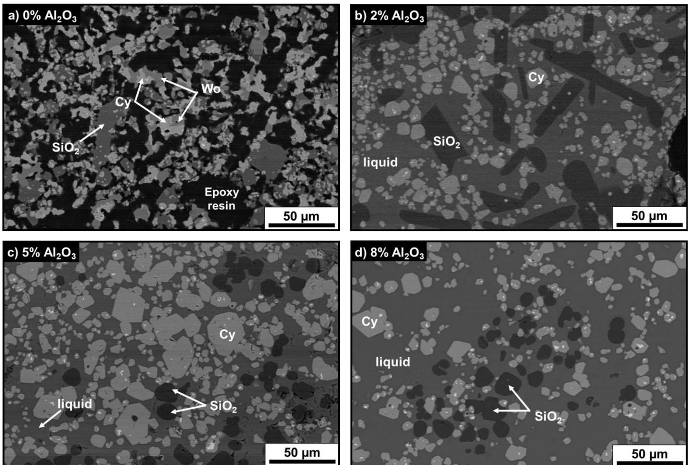
**Figure 3.** SEM micrographs (Back Scattered Electrons mode) of  $\text{C}_{22}\text{S}_{70}\text{Y}_8$  samples without addition of alumina (a), and with addition of 2 mol.% (b), 5 mol.% (c) and 8 mol.% (d) of alumina after heat treatment at 1300°C for 260 hours.
