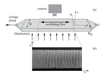
Fig. 1: a) Schematic view of the experimental set-up. b) Top view of a part of the instability pattern. Mean volume fraction  $\phi=0.35$ ; cell gap  $H=0.4\,\mathrm{mm}$ , the cell width,  $W=8\,\mathrm{mm}$ , corresponds to the distance between the two black boundaries.
