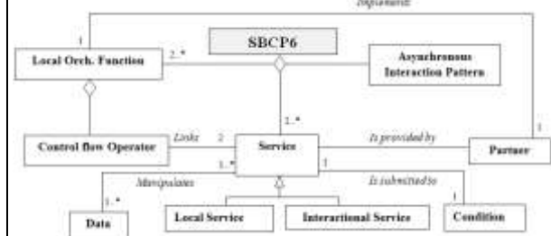
Meta-model of the “Loosely coupled” Pattern
