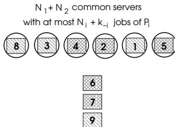
Figure 7: Example of PPR with  $N_1 = 2, N_2 = 4, k_1 = 1, k_2 = 1$ , where jobs of one type can overtake jobs of the other. Jobs 6 and 7 could not enter service because  $P_1$  has reached its limit of  $N_1 + k_2 = 3$  jobs in service simultaneously. Hence, Job 8 belonging to  $P_2$  enters service before them.
