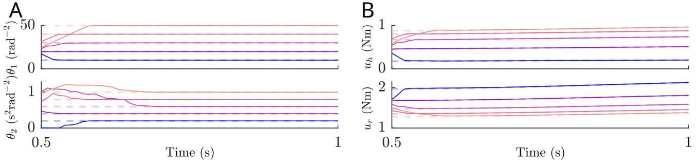
Fig. 2: Estimation of the human cost parameters in simulation. A: The true human cost parameters (position error weight  $\theta_1$  and velocity error weight  $\theta_2$ ) are dashed lines and the estimated parameters are solid lines. B: The true Nash equilibrium torques are dashed lines and the torques recovered the inverse DG method are solid lines.
