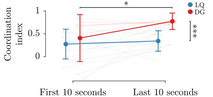
Fig. 8: Human-exoskeleton coordination index during the first and last 10 seconds of the task. Significant effects on the tested conditions are represented by \* if  $p < .05$  and \*\*\* if  $p < .001$
