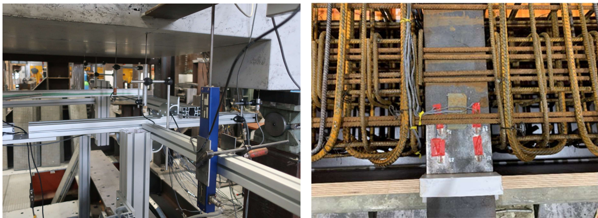
Figure 9: Strain gauges (dimension in mm).
