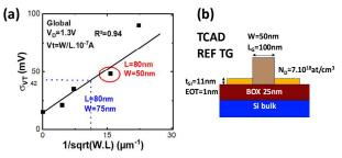
Fig. 4: (a) Experimental pelgrom plot measured for TG-JL nMOS (global variability). (b) REF structure for TCAD simulation with the defined process parameters.
