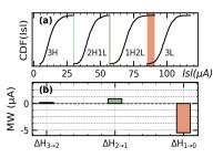
Fig. 6: Scouting logic results with Light Typical SET on three layers represented according to (a) current distributions and (b) Memory Windows values between current distributions, @ Vsl=0.5V.
