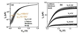
Fig. 3: (a)  $I_D$ -V<sub>G</sub> curves for W=50nm and L=80nm junctionless nMOS at  $V_D$ =1.3V. (b)  $I_D$ -V<sub>D</sub> curves for W=50nm and L=80nm.
