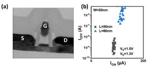
Fig. 2: (a) TG-JL TEM cross-section of JAM (N+-N-N+) transistors. (b)  $I_{OFF}$ - $I_{ON}$  for W=50nm and L=60nm and 80nm.
