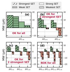
Fig. 8: MW and overlap as a function of SET conditions, on a pillar of four layers, with one (a) to four (d) activated layers @ Vsl=0.5V.
