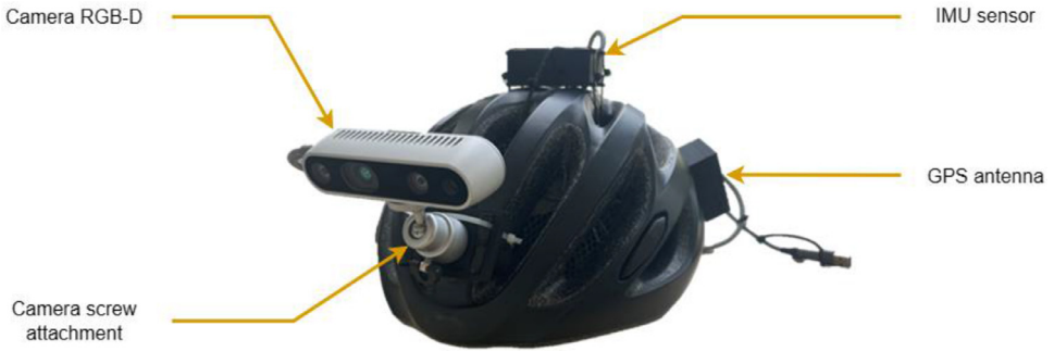
Fig. 5. Experimental acquisition setup.
