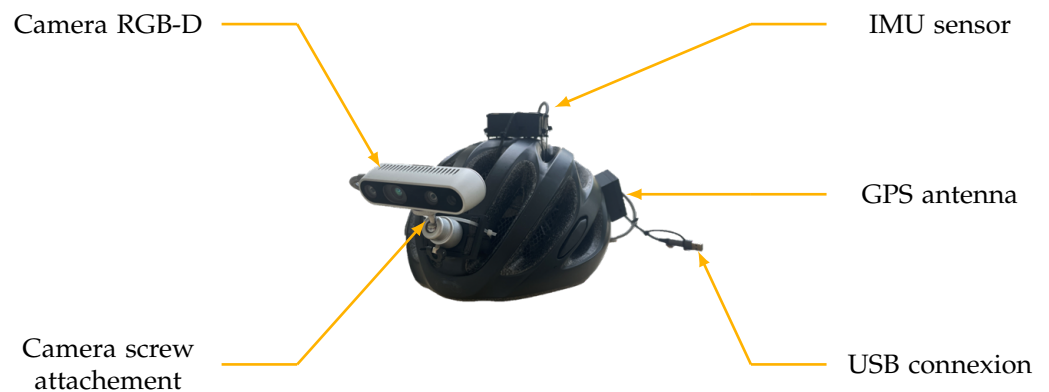
Figure 10. Photography of the acquisition system.
