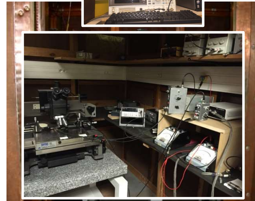
Faraday shielded room (LF noise)
