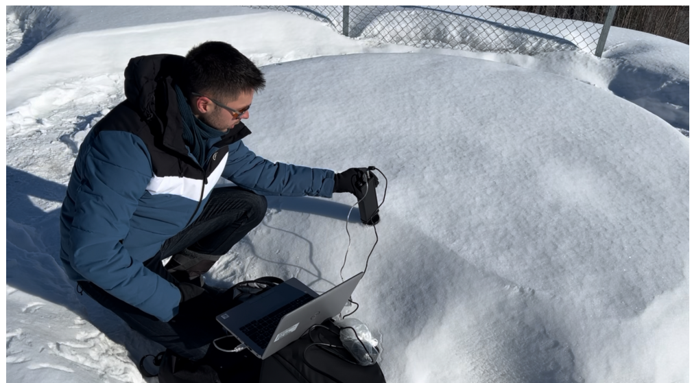
Figure 4. In situ setup to acquire reflectance profiles using the TLS850 for one of the three snow scenes.
