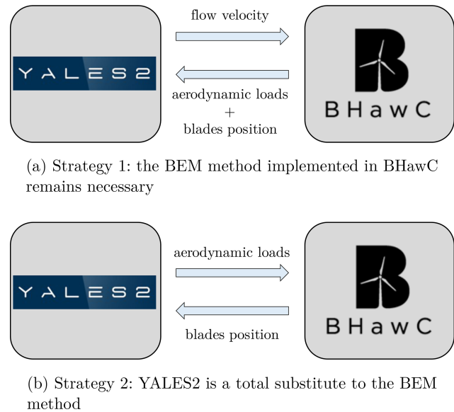
Figure 3. Possible strategies to adopt for the coupling between YALES2 and BHawC. The second one was finally retained because it is more generic.
