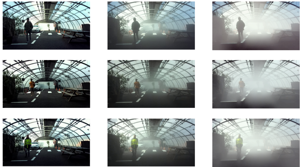
Figure 12. Left: Clear weather images, Middle: Artificial fog produced in PAVIN fog and rain platform, Right: Fog numerically simulated with visibility values of the tests. On the two right columns, from top to bottom, the medium fog visibility values are, respectively, 19, 23, and 26 m.
