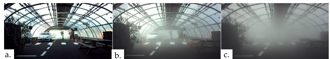
Figure 6. Three weather conditions for a daytime configuration of the scene with (a) clear weather CW, (b) medium fog MF, and (c) dense fog DF.
