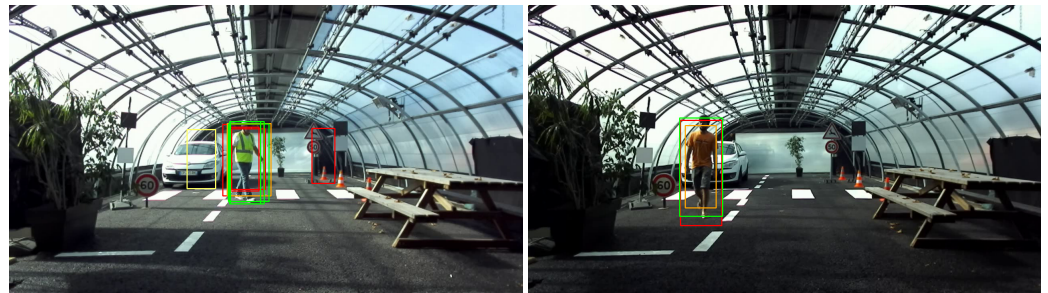
Figure 5. Example of YOLO detections on two clear weather images with different pedestrians. Colors: Green is for confidence > 0.9 , yellow is for 0.9 > \text{confidence} > 0.7 , orange is for 0.7 > \text{confidence} > 0.5 , Red is for 0.5 > \text{confidence} > 0.3 .
