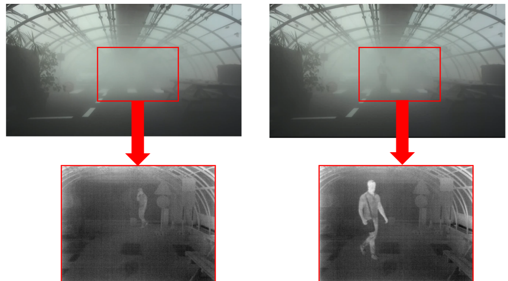
Figure 7. Examples of the field of view of the ZED 2I stereoscopic camera ( top images) with a synchronized field of view of the thermal camera inside the red rectangles ( bottom images).
