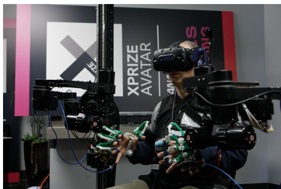
Fig. 5 An Operator judge controls the Team SNU avatar robot using a head-mounted display (HMD), force feedback arms, and haptic gloves during Finals.
