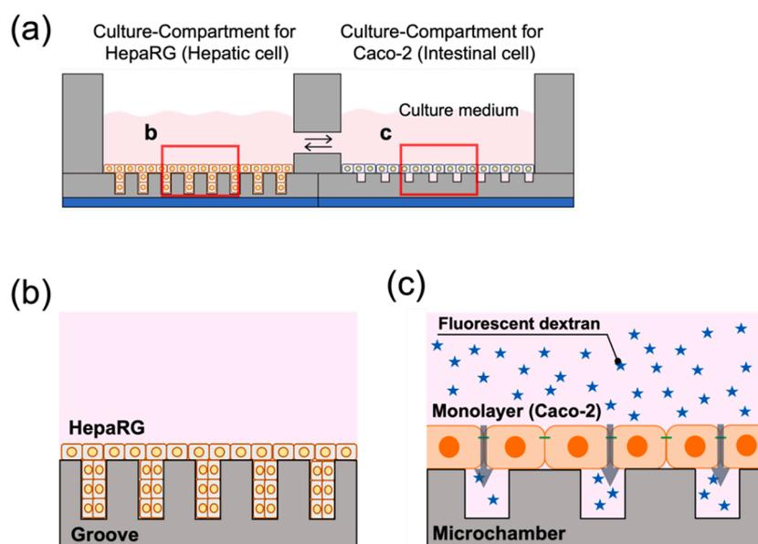
**Fig. 1.** (a) Schematic of the device cross-sectional view showing the microstructures and geometric distributions of liver (HepaRG) and intestinal (gut) (Caco-2) cells. (b) Liver cells cultured in microgrooves. (c) Intestinal cells cultured over microchambers. The paracellular permeability was evaluated by measuring the fluorescence intensity in microchambers emitted by the accumulated fluorescent marker molecules. All illustrations are drawn not to scale.
