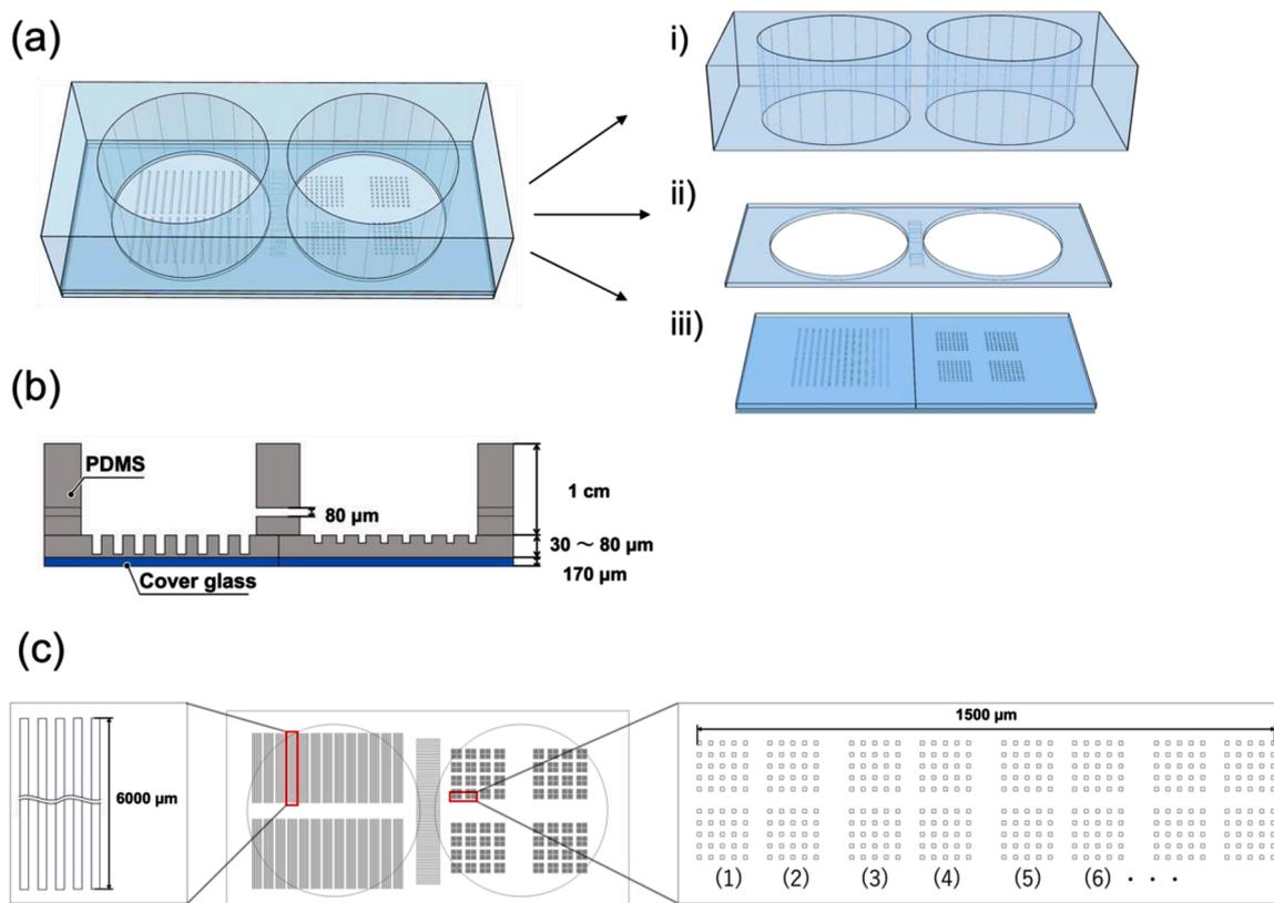
**Fig. 2.** (a) Schematic of the three-layered PDMS construction of the gut-liver co-culture MPS. (b) Cross-sectional view of the assembled co-culture device showing the major dimensions of the device. (c) Actual design of microstructures in the layer (iii). Local parts of the grooves and arrays of microchambers are enlarged on the left and right, respectively. Microchambers at different locations were used for the distance-dependent evaluation of the paracellular permeability.
