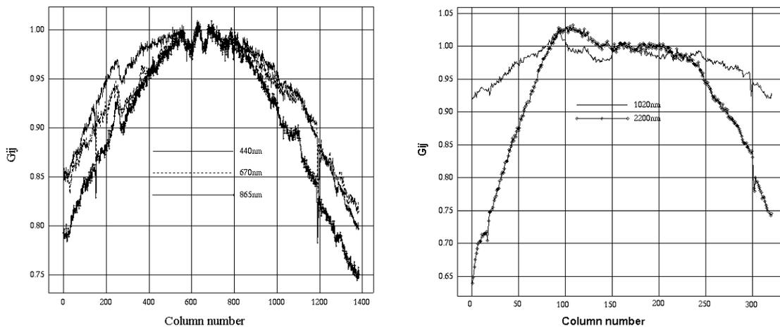
**Figure 6.**  $G_{ij}$  coefficient for a horizontal section, at (left) 440, 670 and 865nm and (right) 1020 and 2200 nm as a function of the pixel column number.
