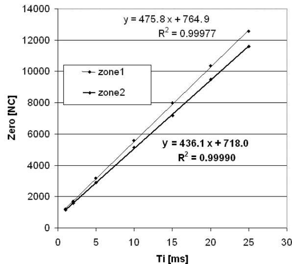
**Figure 4.** Variation of the dark current in two different zones of the SWIR matrix
