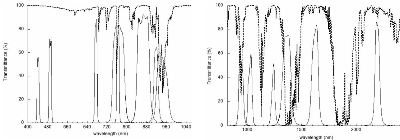
**Figure 2.** Spectral wavelengths of the VIS-NIR (left) and SWIR (right) part of OSIRIS. The dashed line corresponds to the atmospheric transmittance is plotted
