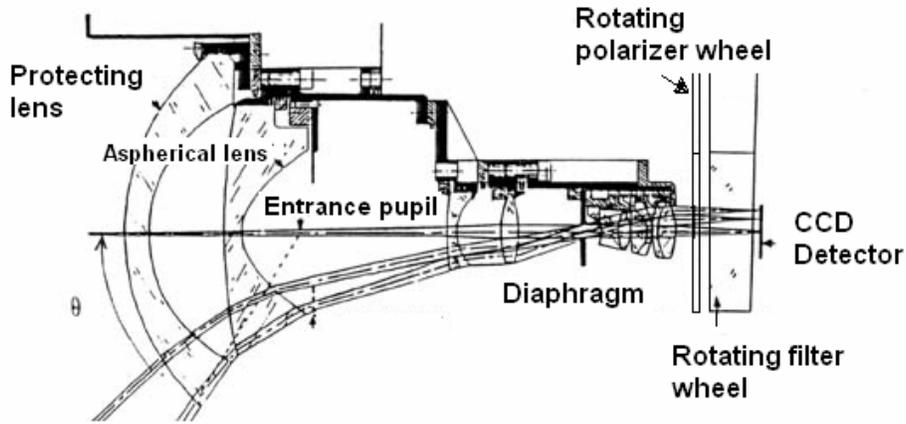
Figure 3. OSIRIS visible lens
