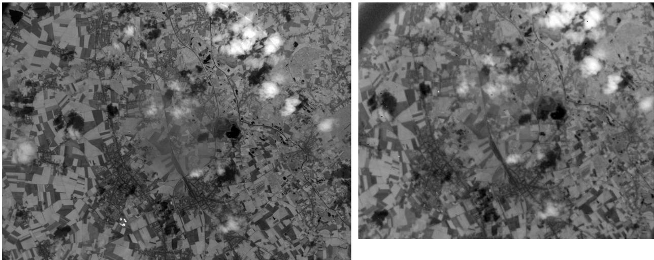
**Figure 8.** Normalized radiances acquired during EUCAARI flight on May 21, 2008 at 940 nm with the VIS-NIR (left) and at 940 nm with the SWIR (right).
