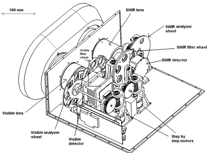
**Figure 1.** Mechanical scheme of OSIRIS instrument
