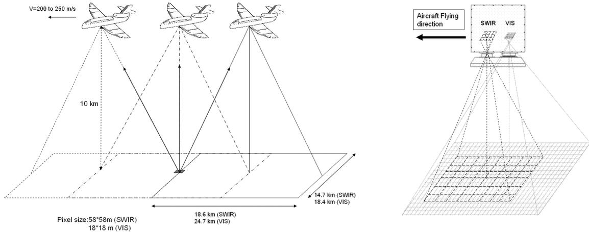
**Figure 7.** (left) OSIRIS multidirectional viewing principle and swath and (right) orientation of the instrument on the aircraft
