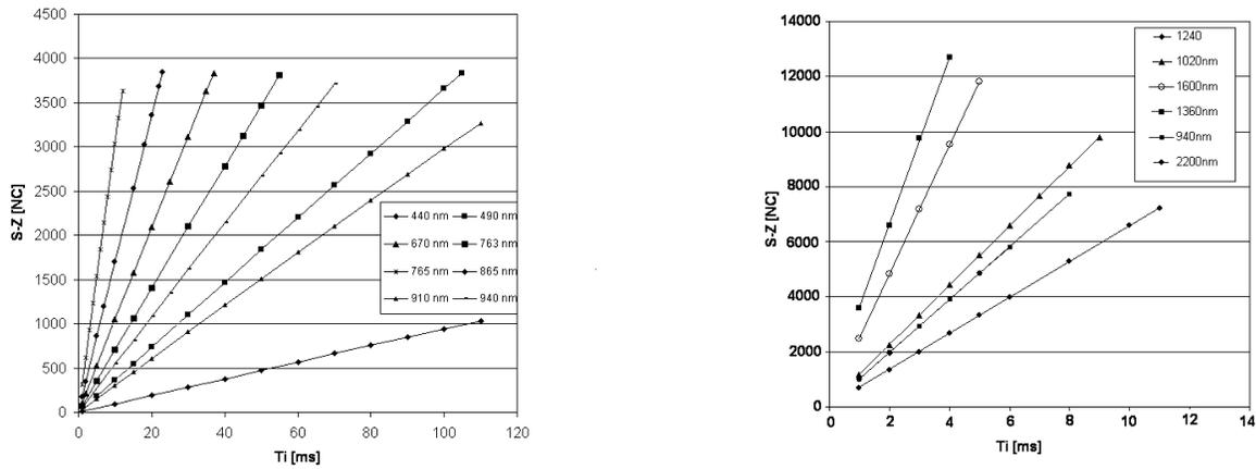
**Figure 5.** Variation of the signal as a function of the integration time for (left) the 8 VIS-NIR channels and (right) the 6 SWIR channels.
