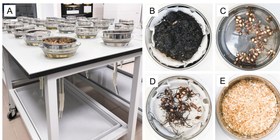
Fig. 5 Nematode tests: A Using the Baermann funnel technique. B Soil. C Stems. D Roots. E Mixture of soil and PWN-infested sawdust
